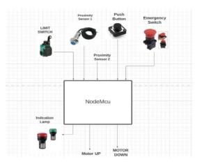
The above picture shows the basic architecture/block diagram of the project. The push buttons are used for starting, stopping and reversing the direction of the motor. Proximity sensors are used for sensing the shutter. Limit switch is used for maintaining the speed of the motor. The output consists of moving the motor up, down and indication lamps. The indication lamps will be used for indication when the motor is turned on or is stopped.
