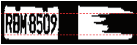
Figure 2.3: Eliminating the upper and lower borders by horizontal projection.
