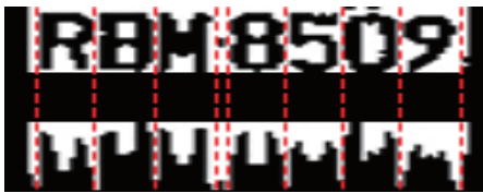
Figure 2.4: Separating characters by vertical projection.
