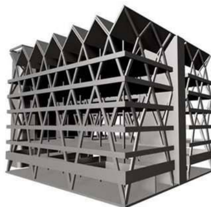
Figure 1- Inclined Intersecting Member Model
