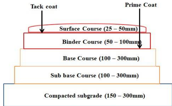
Natural Subgrade Fig 7: Pavement Composition
