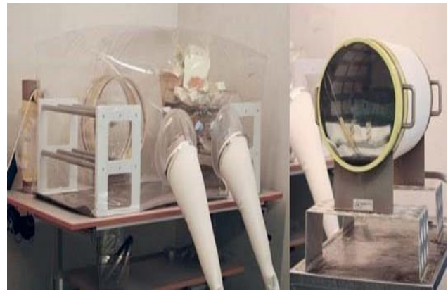
Figure 2 : (A) Isolator for housing germ-free mice. (B) Sterilizing cylinder.
