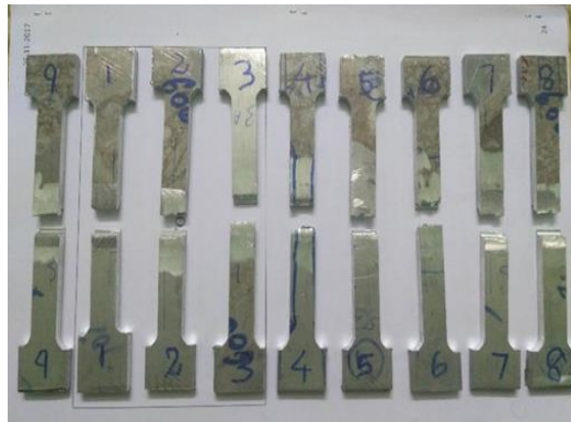
Figure 5.2 Specimens after tensile test
