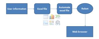
In the DFD level 1,ThisExcel sheet contains the details of students marks, which is to be uploaded in ecampus. The students marks will be automatically updated into the web portal. The robot does the operations instructed by the user.
