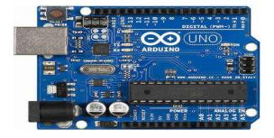
The Arduino Uno is a microcontroller which is based on the ATmega328. Arduino is classified with 14 digital input/output pins, 6 analog inputs, a 16 MHz ceramic resonator. It also has a USB connection, along with a power jack, an ICSP header, and a reset button. It support the microcontroller to be simply connected to a computer with a USB cable or battery to get started. The Uno differs from all preceding boards and does not use the FTDI USB-to-serial driver chip.
