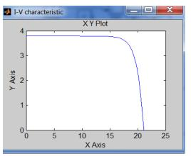
Fig. 9(a) I-V Characteristics of PV module
