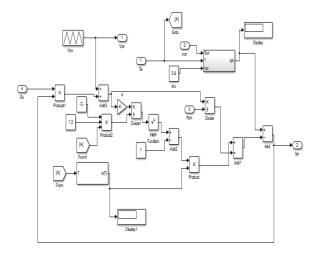
Fig. 6 Modeling of PV module
