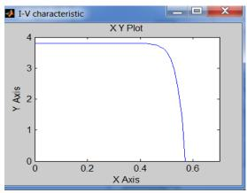
Fig.8(a) I-V Characteristics of PV cell
