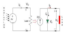
Fig 1: PV Cell with a Load and Its Simple Equivalent Circuit
