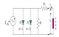
Fig. 3 More Accurate Equivalent Circuit of PV Cell.
