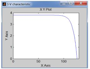
Fig. 10(a) I-V Characteristics of PV Array
