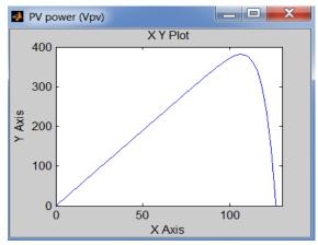
Fig. 10(b) P-V Characteristics of PV Array
