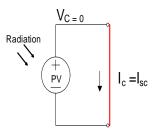
Fig. 2 (a) Short Circuit Condition of PV cell
