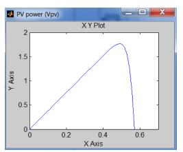
Fig.8(b) P-V Characteristics of PV cell
