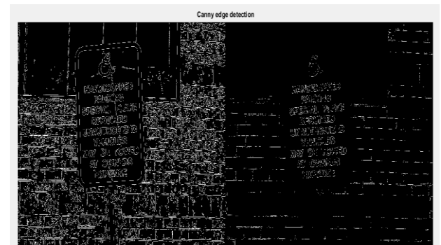
Figure 6: Canny edge detection of the original input image
