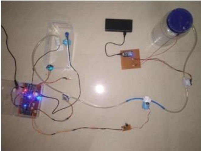
Figure 6 Experimental setup of IoT based real time water quality and monitoring system
