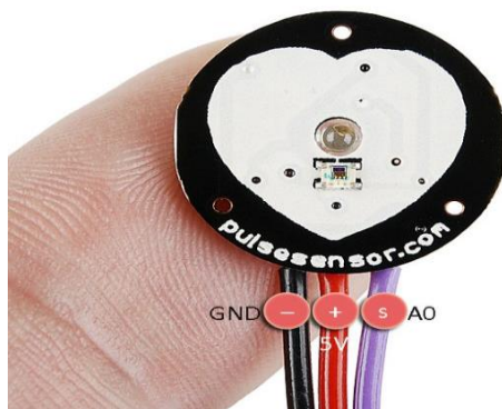
Fig3.2 shows the structure of Heartbeat sensor
