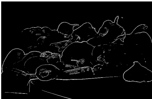
Fig.6 Robert operator with feedback
