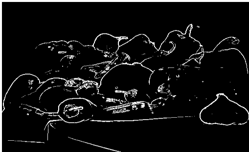
Fig.5 Robert operator without feedback
