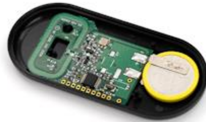
Figure 1. m130 Active RFID asset tag from RF Code
