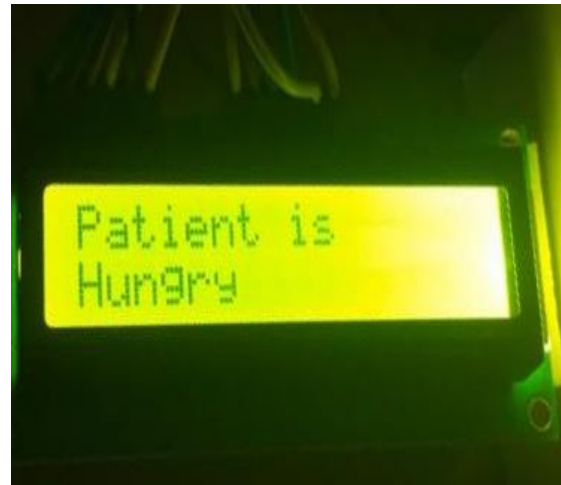
Figure 6.LCD displaying the message “hungry”, which is recognized through hand gesture
