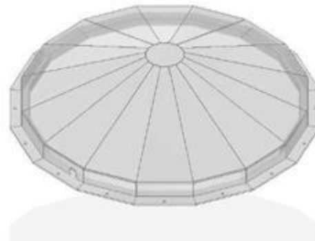
Fig. 4. Glass frame of experimental setup
