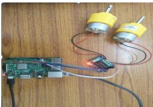
Figure 5.3 Interfacing of DC motor
