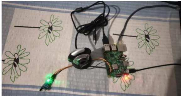
Figure 5.1 Interfacing of IR Sensor and Camera
