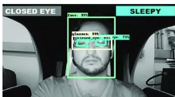
Figure 5 (c): Photograph of combination of Haar classifier and Template matching method.
