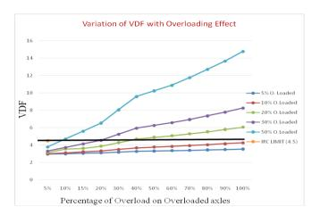
The variation of these values shown in above figure says that it is not increasing exponentially rather increasing nearly linearly because of the assumptions made for this case. Also, between 30% and 50% overloaded axles, at high overloads, the VDF values are nearly doubled. This shows how overloading will be a critical concern for higher overloads.
