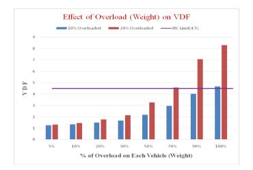
Also, when the percentage of overloaded vehicles is kept constant and percentage of overload on overloaded axles is varied, same result is noticed. Vehicle Damage Factor is increasing with percent of overload on axles. But it is nominal in initial stages of overload such as 5%, 10% for less number of overloaded vehicles. But it has shown a sudden hike with the percentage of overload for large proportion of overloaded axles which are depicted in figure below
