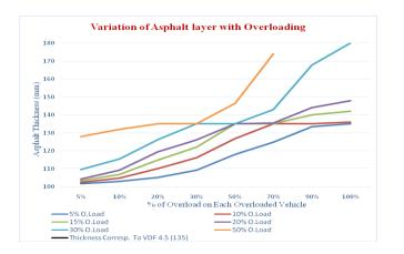
So, it can be inferred that the thickness of asphalt layer is increasing in greater amount as the overload and proportion of overloaded axles increasing.
