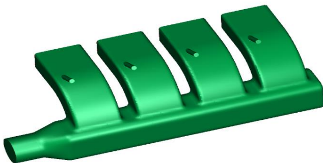
Intake manifold Core
