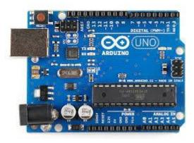
Arduino is an electronics device based on hardware and software. It uses microcontroller Atmega328.It has both Analog and digital pins. All the sensors are connected to Arduino. The Analog pins are used to connect with the sensors. It reads the input light of a sensorand converts it to output. Arduino collects all the data from the sensors and sends them to Database storage through MCU Node.
