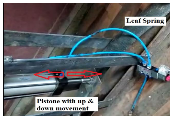
Fig. (10.2): Solenoid Valve/Pistone reciprocates up and down, acting point load of different magnitude on composite leaf spring.
