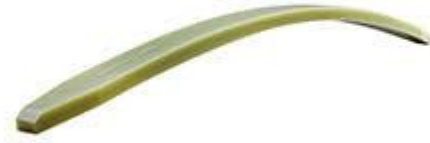
Fig. (3.1): Composite leaf spring structure formed after molding/hand layup method
