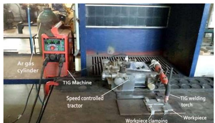
Fig. 4: Experimental set-up for TIG welding
