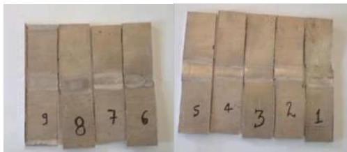
Fig. 5: Welded specimen 1-3 performed with the welding speed of 3 mm/sec. and welding current 120, 130 and 140 A and gas flow rate of 8 l/min., Welded specimen 4-6 performed with welding speed of 3.5 mm/sec. and welding current 120, 130 and 140 A and gas flow rate of 9 l/min. and Welded specimen 7-9 performed with welding speed 4 mm/sec. and welding current 120, 130 and 140 with gas flow rate of 10 l/min. respectively.
