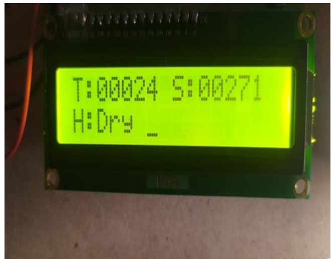
Fig : A 16 x2 LCD Display displaying the temperature, smoke and humidity
