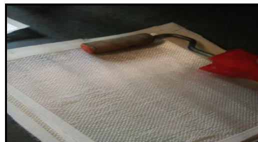
Fig. 4. Procedure by hand layup method
