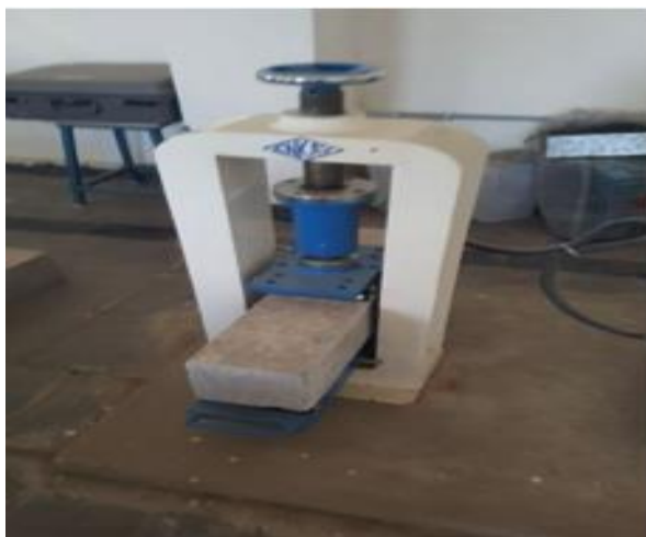
Fig.2 showing the testing of Flexural Strength specimens.
