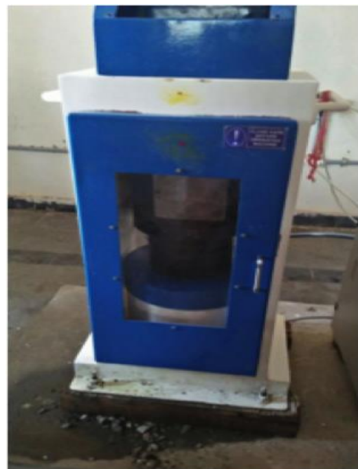
Fig.1 showing the testing of the cube specimens in the compressive s=testing machine.
