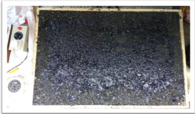
Snow Melting System with Temperature Controller.
