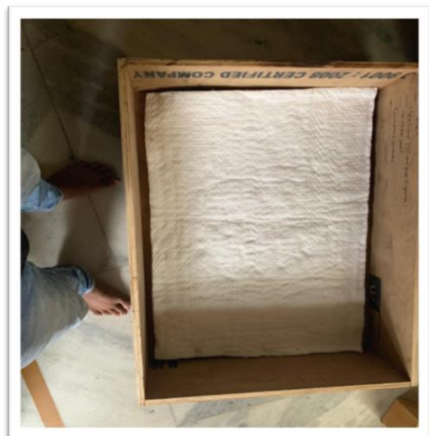
Step 3 :- Layer of Insulator ( Silicon Wool ).
