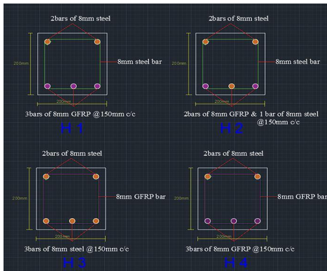
Fig 2. Reinforcement detailing of Hybrid beam
