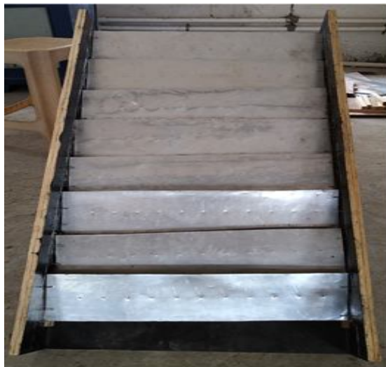
Fig. 4: Aluminum sheet plates installed in Heating Cabinet
