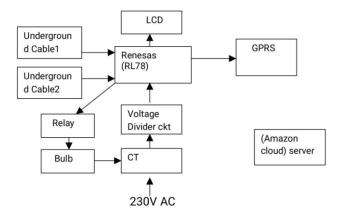
The figure represents the block diagram of IOT Based 0.4 Underground Cable Fault Detection.. It consist of hardware components such as renesas microcontroller, LCD, Voltage divider circuit, bulb, relay, current transformer, server, cables.
