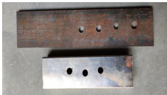
Fig: 5.2 After drilling operation on the work piece
