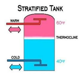
The storage volume with this type of system is reduced relative to other systems, because the dead water volume is relatively low and the energy efficiency relatively high. Performance of the stratified thermal storage tank is more effective when compared to mixed storage. To increase the degree of stratification baffles can be used effectively. The performance of the thermally stratified storage tank with baffles and without the use of baffle plate is analysed.
