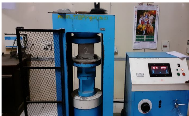
Figure 5.1 Compression test on cube
