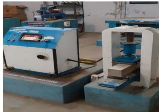
Figure 5.7 Flexural test on Prism
