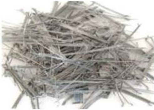
Fig 2: Steel Fibers with hook end.
