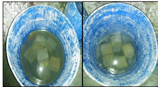
Figure 1: Specimens curing in 5% H 2 SO 4 (acid attack test) and 5% Na 2 SO 4 (sulphate attack test)
