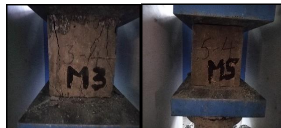
Figure 5: Compression test under progress
