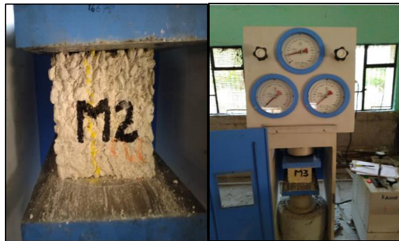
Figure 2: Compression test under progress after total immersion of 56 days
