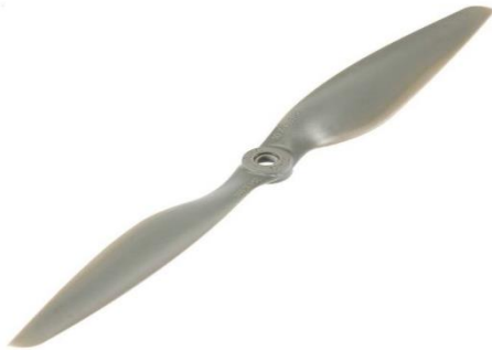
Figure 3- 10 x 4.5 inches Propeller
