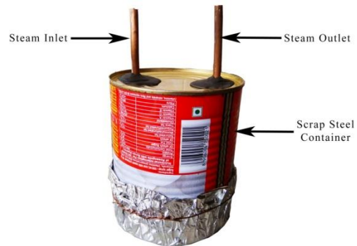
Fig 3.5: Fabricated Steam Chamber
