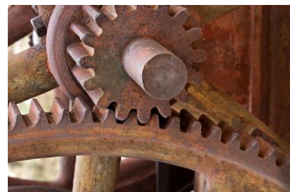
Fig-3 Corrosion Products on steel Surface
