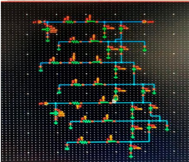
Fig. 7. Four lines of RLC interconnect model with alternative an input.
