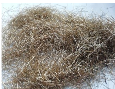
Fig 1: Brass coated micro steel fibers
