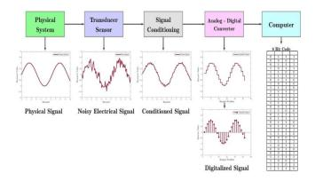
DAS is used for signal conditioning of the signal received from sensor and providing sequential filtered output signal to the controller.
