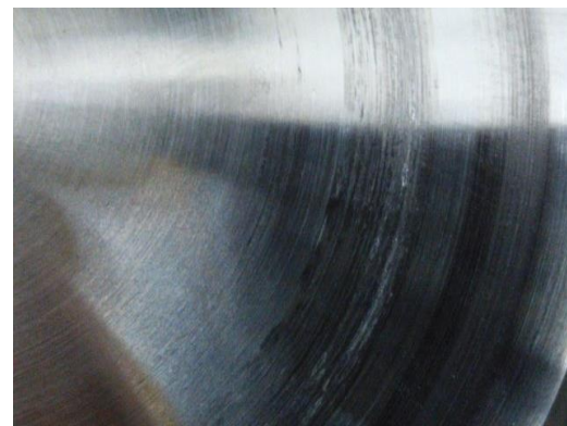
Fig 3. Track of the Specimen after wear test
