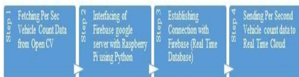
Fig. 2: Systematic flow diagram to illustrate the image processing operations for obtaining the count the present vehicles
