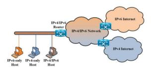
Tunneling approach is a mechanism that employs the existing IPv4 infrastructure to carry out the IPv6 traffic. The tunneling approach is useful when two IPv6 networks are separated with an IPv4 network. When an IPv6 packet from the first IPv6 network wants to reach the other IPv6 network, it will be encapsulated into IPv4 packets and transmitted throw the IPv4 network to its destination.
