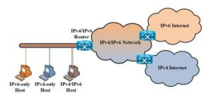
Dual-Stack approach is the idea of implementing the IPv4 and the IPv6 protocol stacks in the dual stack devices. Also, providing the connectivity to both IPv4 and IPv6. The dual stack devices could be any device that connected to the internet (i.e. routers, infrastructure devices, and end-user devices)
