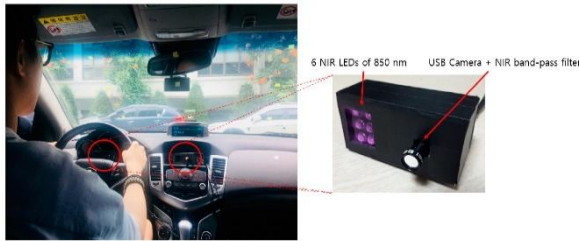
Figure 5. Camera on the stereo (for face recognition)
