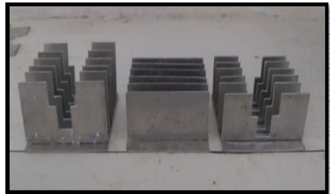
Fig.3 Assembly of Rectangular fin array
