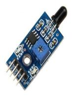
Flame sensor is connected with a BLYNK app and will show the notifications if a tree is under fire.
