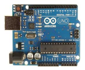
Arduino uno is an open platform used for building electronic projects. It consists of both physical programmable board and a software, here you can write and upload the code to the physical board.
