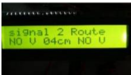
Fig. 4: Information Related to the Density of the Traffic on the Road. Since the Output is Displayed for the 2nd Sensor- Density on the Road is Medium
