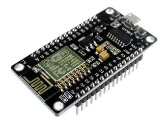
The most basic way to use the ESP8266 module is to use serial commands, as the chip is basically a WiFi/Serial transceiver. However, this is not convenient. What we recommend is using the very cool Arduino ESP8266 project, which is a modified version of the Arduino IDE that you need install on your computer.
