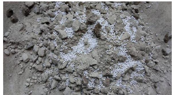
Fig. 4 mixing of aggregate, Fly ash and EPS
