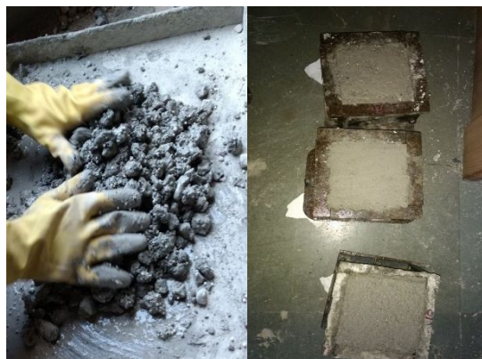
Fig. 6. Hand mixing of concrete and filling it in the mould
