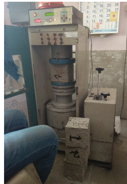
Fig. 7. Specimens at the time of compressive testing in CTM machine
